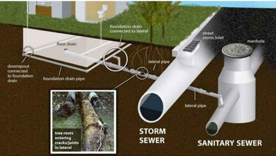
The lateral pipe directs wastewater to the sanitary sewer under the street. Source: MMSD
