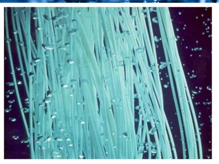
Figure 2. Hollow-fiber membranes (Image from GE/Zenon)
