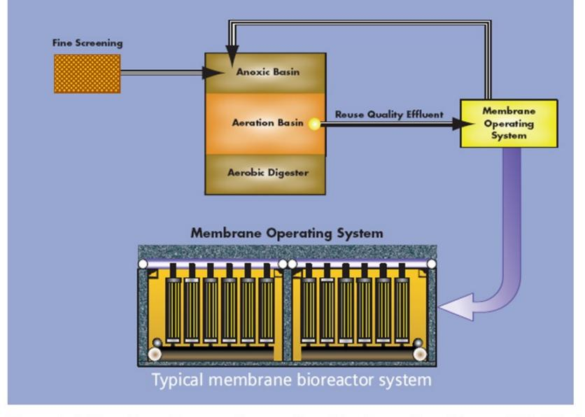
Figure 4. External membrane system configuration (Image from Siemens/U.S. Filter)
