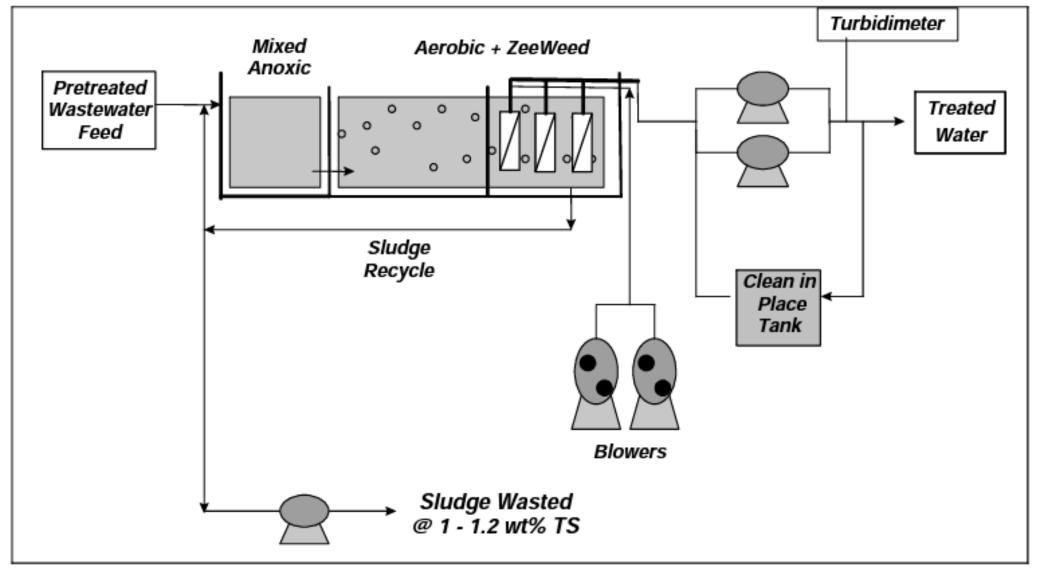
Figure 3. Immersed membrane system configuration (Image from GE/Zenon)
