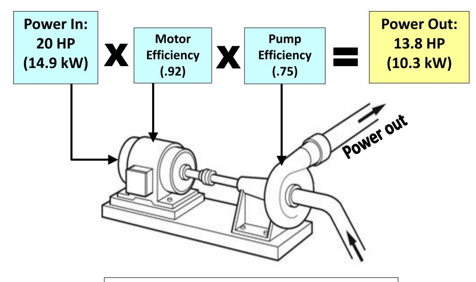
Overall Wire-To-Water Efficiency in This Example = .69 OR 69%
