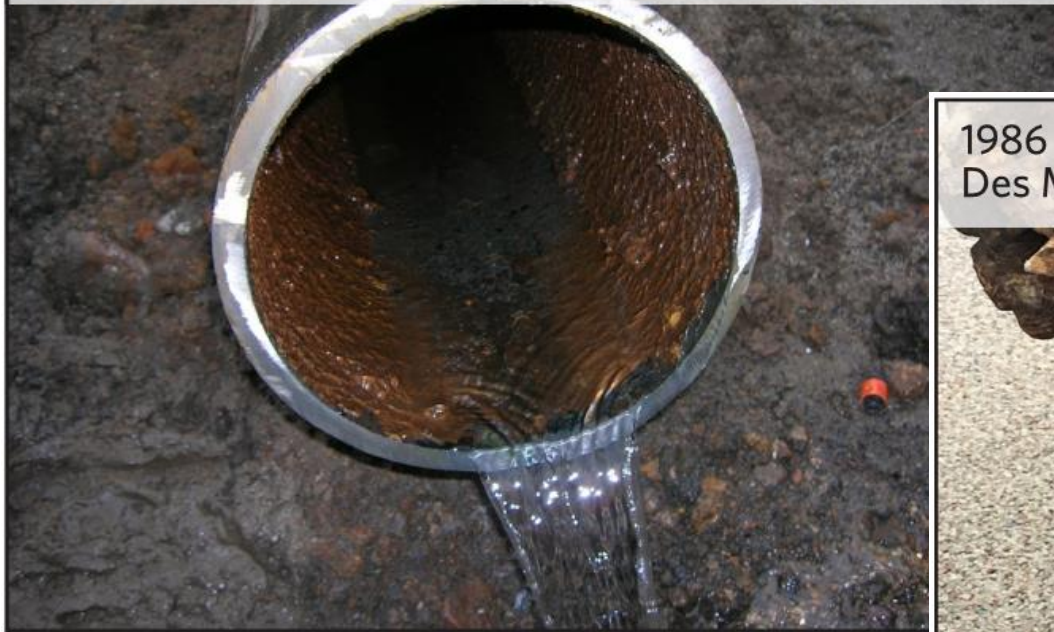
1896 - 12" Cast Iron Water Main Des Moines, Iowa
