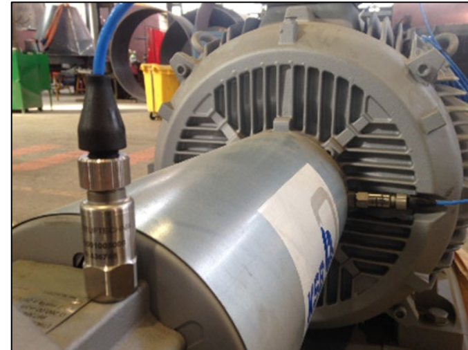
Vibration analysis: An increase in vibration over time can indicate bearing, impeller, or alignment problems
