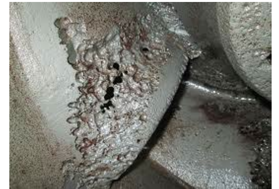
Cavitation damage to the impeller
